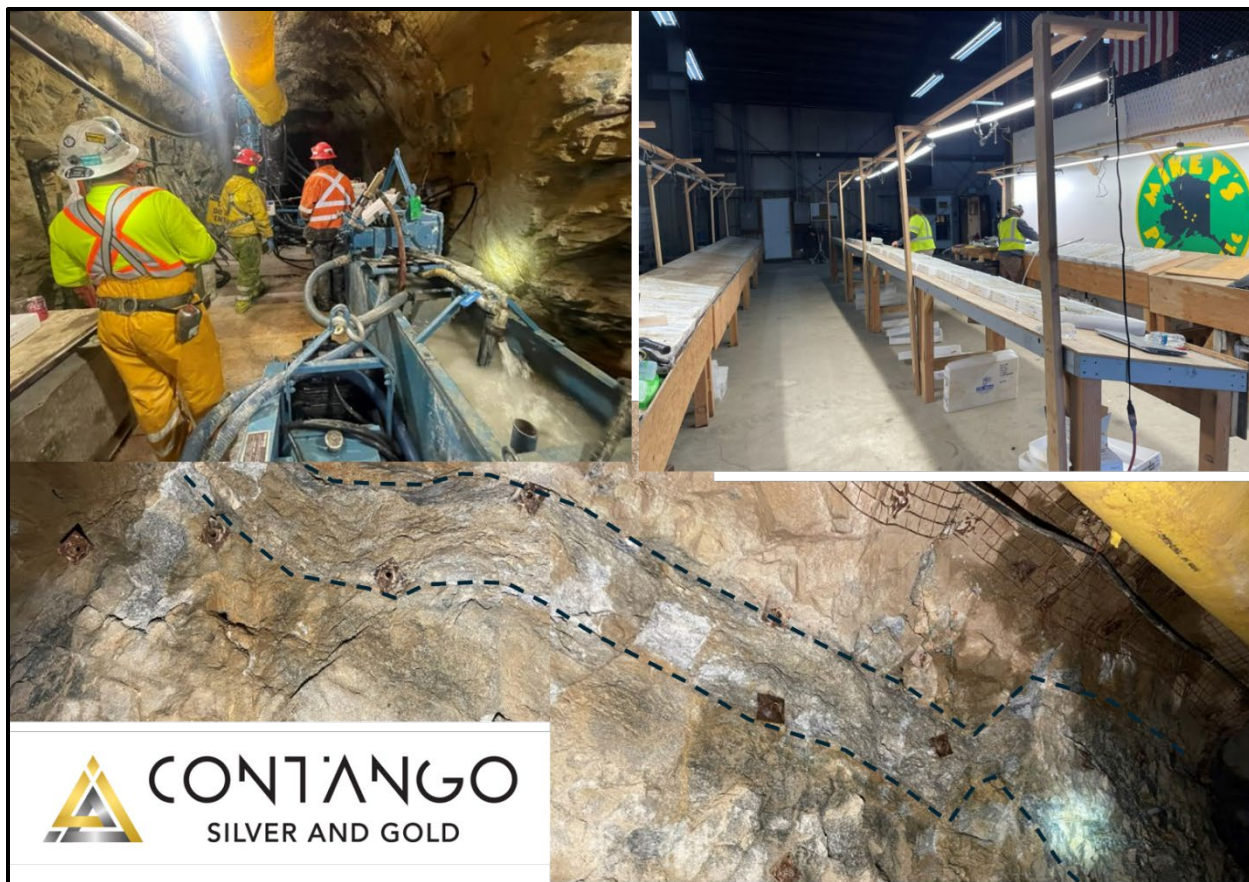
Figure 1. Lucky Shot exploration activities. Upper left: drilling station in the West Drift Extension. Upper right: the new core shack at the Lucky Shot Outpost. Lower image: the KM vein exposed in the West Drift Extension.
