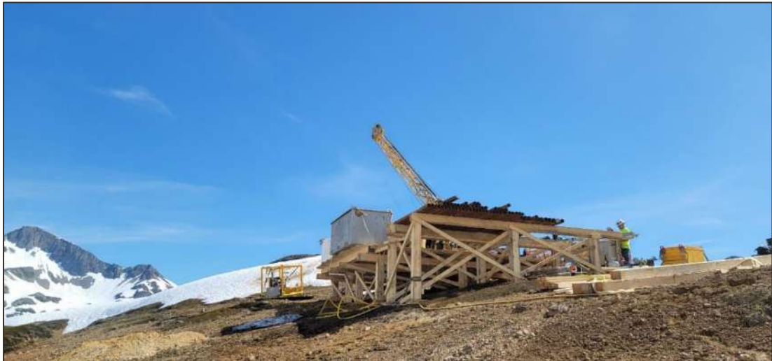
Plate 10.2 Ruen's Modified Longyear LF-70 Drill Rig on Hole DC21-010 at Middle Difficult Creek
